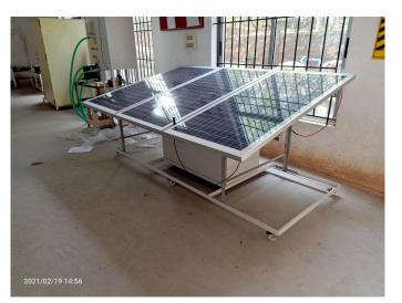
Solar Photovoltaic water pumping system
