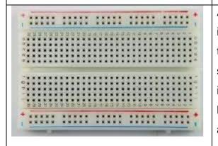
A breadboard is a solderless gadget for impermanent model with hardware and test circuit plans. Most electronic segments in electronic circuits can be interconnected by embeddings their leads or terminals into the openings and afterward making associations through wires where suitable.
