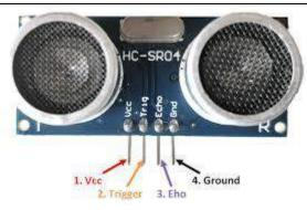
A ultrasonic sensor is an electronic gadget that gauges the distance of an objective article by discharging ultrasonic sound waves, and converts the reflected sound into an electrical sign. Ultrasonic waves travel quicker than the speed of discernible sound (for example the sound that people can hear).
