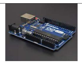
Aurduino Uno Microcontroller: It is an open source with both equipment and with programming drive 8 bit ATmega328 a low force CMOS regulator dependent on RISC design .It has best with assortment of decisions completely static activity and self programmable blaze program memory in the framework. It very well may be fueled utilizing USB link from PC either an AC mains supply.
