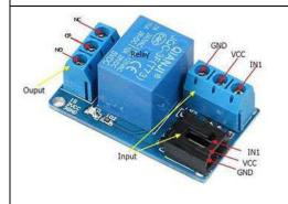
Relay: It is used to connect the valves to the
