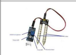
Soil sensor: This dirt sensor identifies the dampness level of soil on field from 20%(wet) - 200 % (dry). It is a circuit board having two tests which detects the dirt status. This sensor will show the volumetric substance of soil and loss of water content because of vanishing. This sensor is converged with the regulator and coded.
